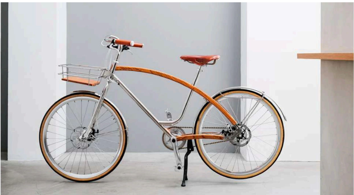
the Craftsmanship Bicycle Project comes from AOI product, which applies the aerospace welding technique, fashioned with used vegetable-tanned leather in places such as handlebars, saddles, and bicycle parts
